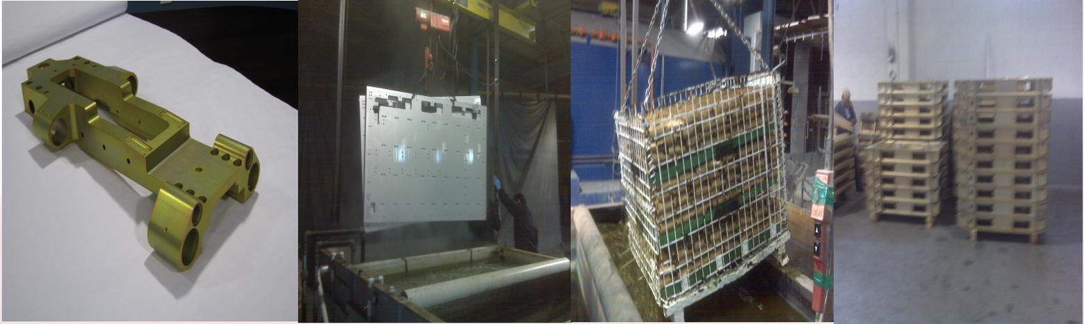
Our Chem Film lines have both large tanks and small ones allowing us to handle the small lots as well as the large runs with both Etch and Non Etch cleaners. Meeting MIL-DTL-5504F Specifications.
