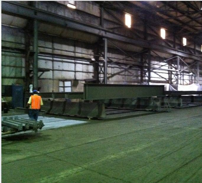
800 Foot Girder bays and lay-down allows for large projects or multiple ones. Supported by 60 ton over head cranes
