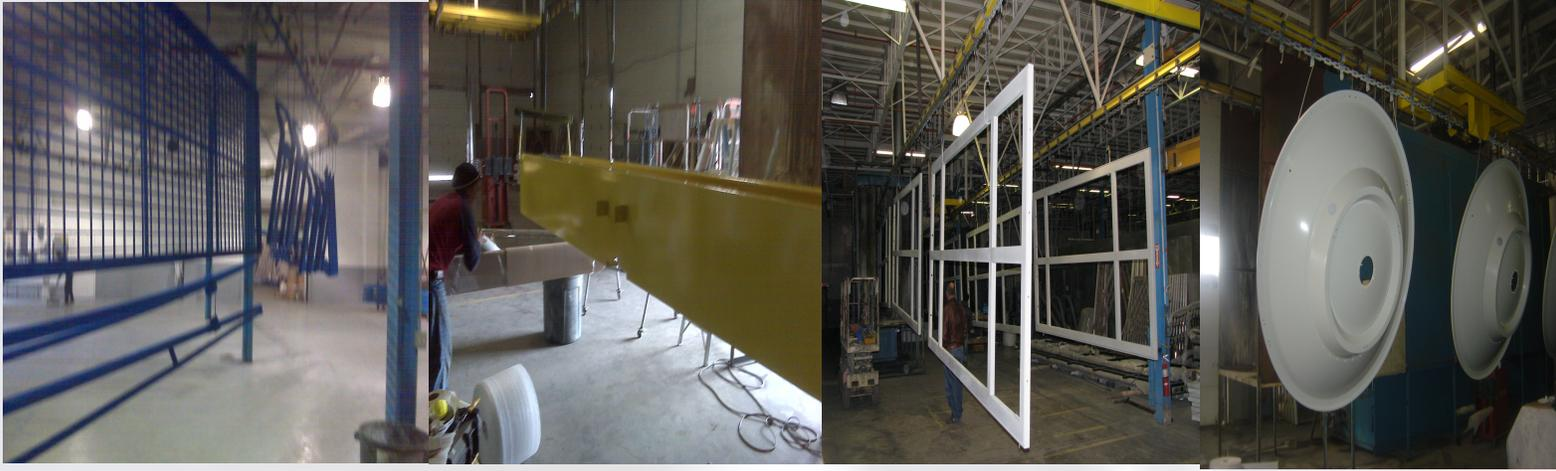
Our Large Powder Line can handle runs of a few parts up to thousands with its large part openings. 3 stage Iron Phosphate and capable of both Powder or Wet finishes it allows the flexibility to handle almost any project size or type.
